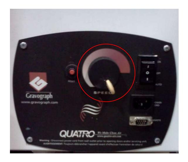
Turn the knob completely counter-clockwise (minimum). When you're done, restore the knob setting to its original position.
