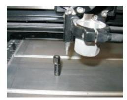
To replace the sensor, simply unscrew the hexagonal portion and screw on the new one.
